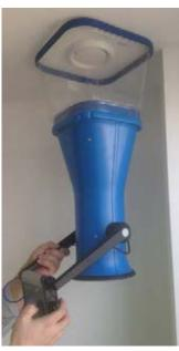
MEASURE AIRFLOW WITH APPROPRIATE DEVICE
